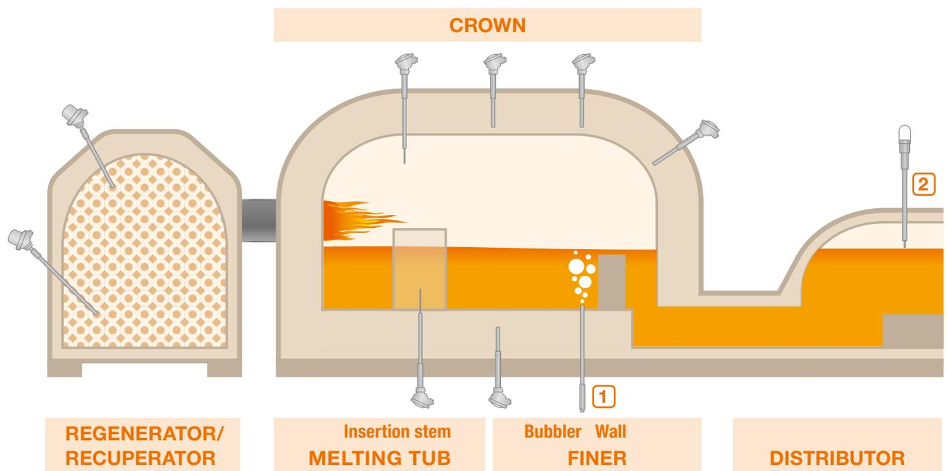
Thermocouples and auxiliary devices in a typical glass manufacturing process can be classified according to their place of use and design.
